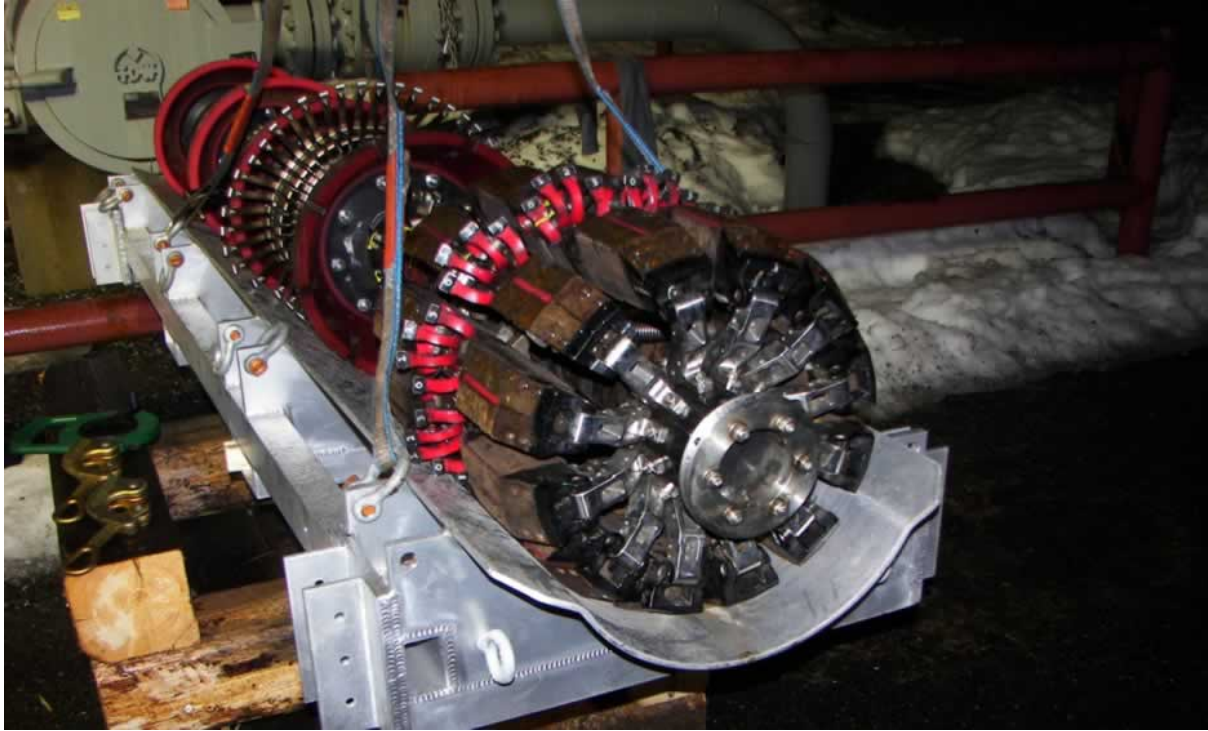
Figure 3 Inline Inspection Device (Smart Pig) used for Integrity Assessment
