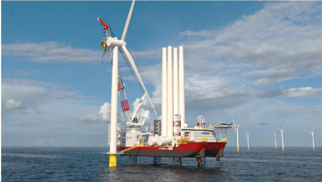
Figure 6.2.1. Mockup of the Charybdis, the first domestically built JA compliant WTIV due to be completed in late 2023 (Dominion Energy).
