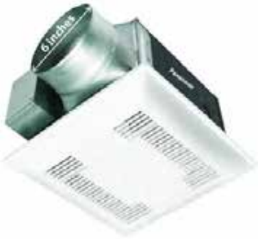
Two- or variable-speed fan: An occupancy sensor toggles between speeds. A 6-inch outlet provides airflow for whole-building ventilation.
