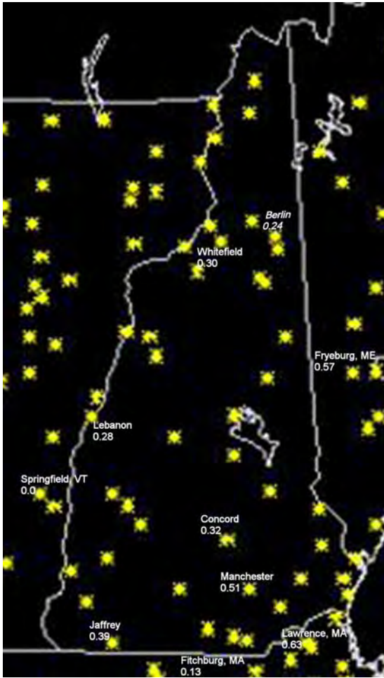
Figure F-5-Weather stations in New Hampshire and the surrounding area and equivalent radial glaze ice in inches.
