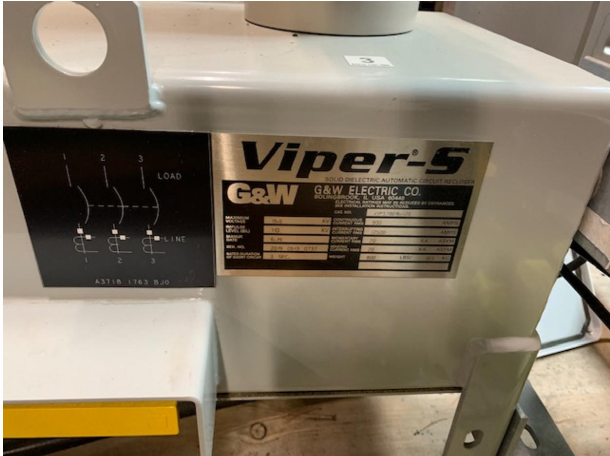
Photo 3 courtesy of PUC Safety Division taken 3/6/2020. Photo inside of the warehouse at the Lebanon Area Work Center. The photos shows the Manufacturer (G& W) Viper S recloser nameplate ratings for the recloser. Specifically 15.5 kV maximum voltage rating, 110 amp impulse loading (BIL), 800 amp continuous current, manufacturing date of 6/2019, interrupting current rating of 12,500 amp, making current RMS 20 amp, 800 pound weight of assembly.
