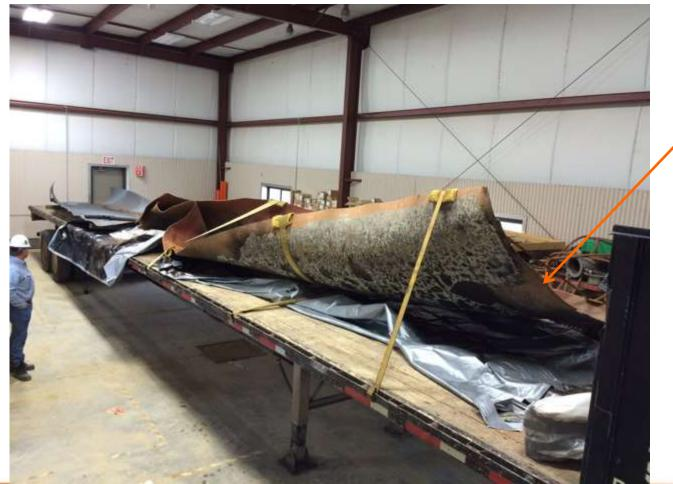
Suspected Origin of Failure
