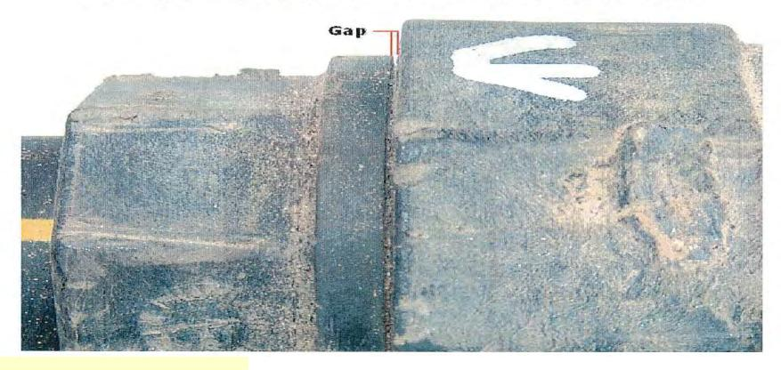
2" Polybutylene SDR 9 (1976) Crack from rock impingement Plunger hole day of investigation
