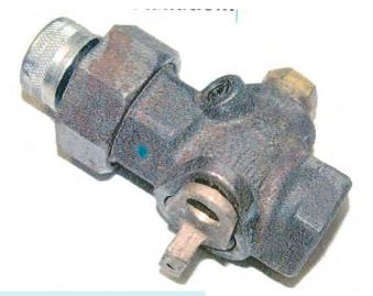
Mueller Insulating Riser Valve: <u>Not</u> caused by over tightening, manufacturers defect.
