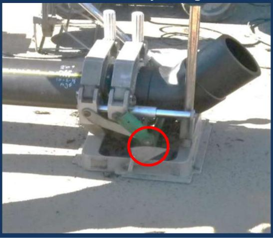
\$10,000 – service installed without 12" clearance
